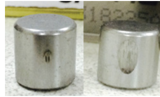
Right Same Timken experiment is performed on metal piece after engine oil after six-month and 15,000km of service. (2010 Honda Civic 1.8, Extreme 0W-30 is being tested)
